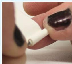
Make sure that the fiber paper posts are just slightly larger in diameter than the brass anchor (1/4") before inserting into mold.
