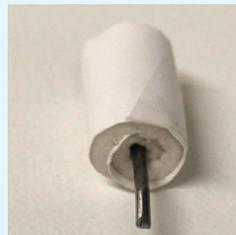
1/8" thick fiber paper cut 1/2" x 1", kiln shelf paper cut 1/2" x 1.25" rolled tightly and held together with a small piece of scotch tape.
