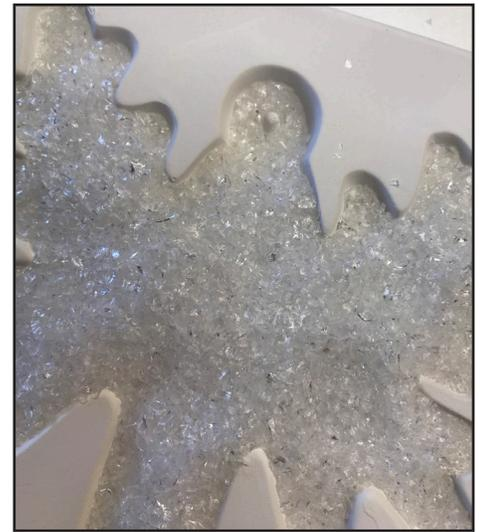
Cover the cavity with F3 Medium Clear frit until the mold holds a total of 96 grams of glass.
