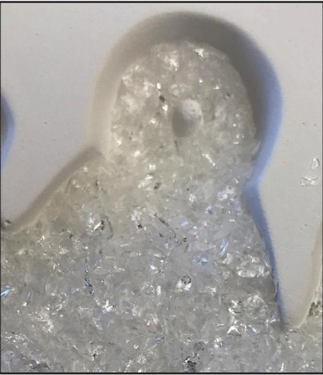
Gently sweep the frit away from the post with a paint brush or similar tool to prevent burrs. Fire the mold using the schedule found in table 1.
